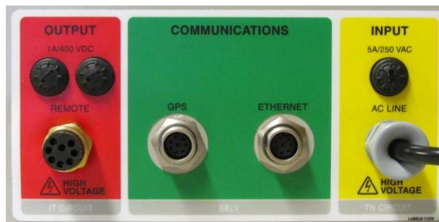
Figure 5-4: 375V Host Interface Operational Connectors
