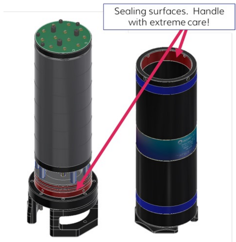
Figure 05: Battery pack sealing surfaces are shown in red
