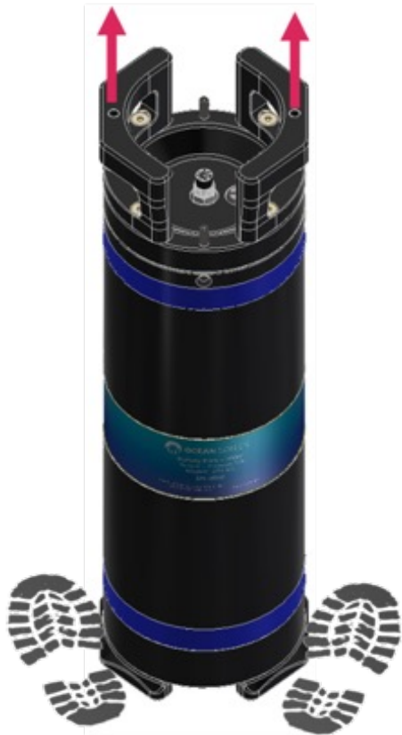
Figure 04: Battery pack showing feet placement for end cap removal
